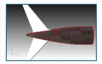
**Step 1:** NLign quickly aligns hundreds of UT scans to a model of the fuselage, aggregating data from multiple fuselage sections in seconds.
