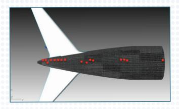
A detailed report was then generated, illustrating the porosity indications as a function of mold tool set. This report clearly showed that the majority of porosity problems along the problem seam were associated with one particular tool set.
